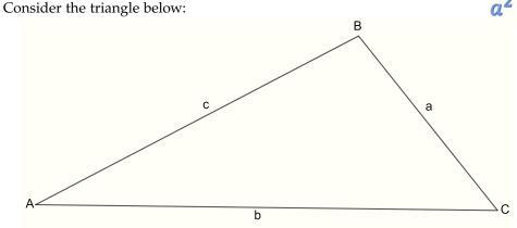
The angles A, B, C are the angles at the vertices A, B, C respectively. The sides a, b, and c are opposite angles A, B, C respectively. The Cosine Rule states:
